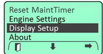
Navigate through the “Display Setup” menu using “⏴” softkey until the “Contrast” entry is highlighted. Press the “➔” softkey to select the contrast parameter setting.
