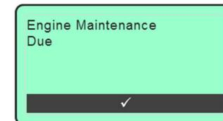
To reset the maintenance timer enter the Main Menu and then scroll to the “Reset MaintTimer” entry using the “↓” softkey. Press the “→” softkey to select the reset maintenance timer menu item.
