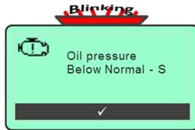
The acknowledge alarm stripe at the bottom of the display prompts the operator to acknowledge the fault. The controller also blinks the red LED fault indicator located above the digital display.
