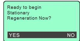
**Continuing** with the regeneration request by selecting “Yes” will command the engine to enter regeneration mode. The control system will display a waiting prompt until the engine acknowledges the manual regeneration state.
