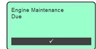
To reset the maintenance timer enter the Main Menu and then scroll to the "Reset MaintTimer" entry using the "↓" softkey. Press the "➡" softkey to select the reset maintenance timer menu item.
