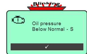
The acknowledge alarm stripe at the bottom of the display prompts the operator to acknowledge the fault. The controller also blinks the red LED fault indicator located above the digital display.
