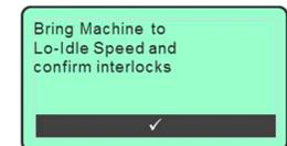
The prompt also reminds the operator confirm that all interlocks have been set. (Note: Interlocks are application specific, are hardwired into the engine harness and are not controlled by the control panel.) The operator must acknowledge this prompt by momentarily pressing the “✓” softkey.
