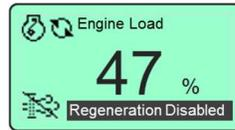
When the operator selects “Allow” the control panel will guide the operator through an interactive sequence of displays to start regeneration.
