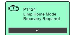
The operator will then be prompted to begin the recovery process or continue to delay the regeneration process. Selecting the “Yes” softkey will proceed with the recovery regeneration process. Selecting the “No” softkey will delay the recovery regeneration process.
