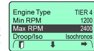
Navigate through the “Engine Settings” menu using “↓” softkey until the “Max RPM” entry is highlighted. Press the “→” softkey to select the Max RPM entry setting.
