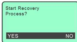
**Continuing** with the regeneration request by selecting “Yes” will command the engine to enter regeneration mode. The control system will display a waiting prompt until the engine acknowledges the recovery regeneration state is active. Should all conditions not be met the control system will display a checklist of items for the operator to review.
