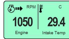
To change the data being displayed press any key to activate the softkey menu. Press the change “U” softkey to access the next data display available.
